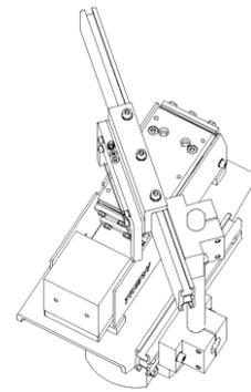
*VH series linear feeders are studied for conveying, handling and accumulation of various kinds of products. They have an electromagnetic vibrating base and their own controller. Accumulation canal is studied case by case to guarantee maximum reliability. If requested, empty and full detector will be provided to synchronize linear feeder with the orientator.*
