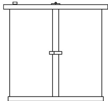
Soundproof covers are used to reduce noise and as protection against injuries. They are projected case by case on the basis of equipment inside it.
