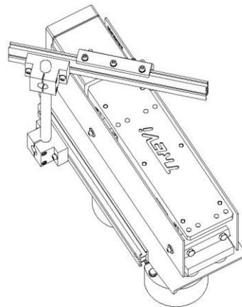
*VH series linear feeders are studied for conveying, handling and accumulation of a wide range of products. They have an electromagnetic vibrating base and their own controller. Accumulation canal is studied case by case to guarantee maximum reliability. If requested, empty and full detector will be provided to synchronize linear feeder with the orientator.*
